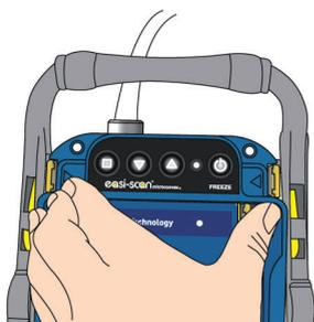
Press the Easi-Scan firmly into place. Make sure that the clips are fully engaged.
